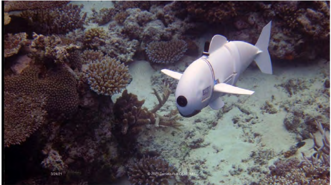
Figure 23. SoFi, the soft robotic fish swimming in a coral [236]. Photo credit: Joseph DelPreto.
